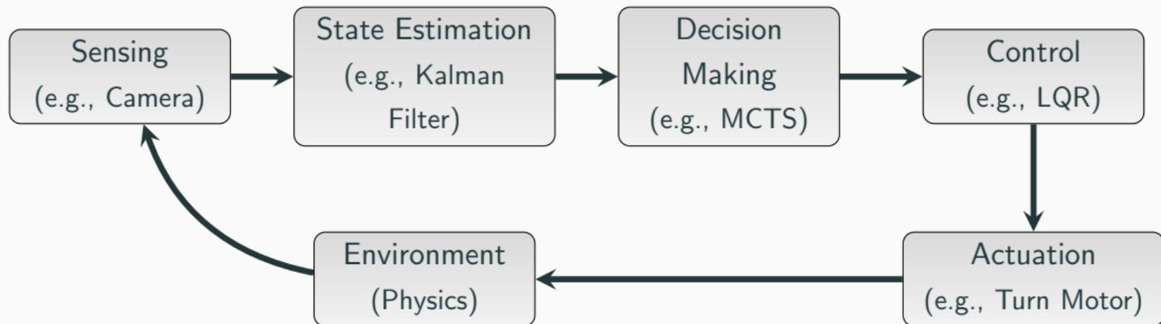
Motion Planning is a **part of decision making**: How to **reach the goal**, **given the state** of the robot and environment, without collisions.
