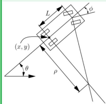
We have  $\mathbf{u} = (s, \phi) \in \mathcal{U}$  and  $\mathbf{q} = (x, y, \theta) \in \mathcal{Q}$ , where  $s$  is the speed,  $\phi$  the steering wheel angle,  $x, y$  is the position, and  $\theta$  is the orientation. The dynamics  $\dot{\mathbf{q}} = \mathbf{f}(\mathbf{q}, \mathbf{u})$  are:
